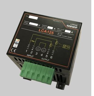
The LCA125 is an active inrush current limiter with a delayed bypass relay ensuring a more efficiency operation compare to a NTC element. It cut-off the current peak in the load at the installations start-up and does not dissipate power when operating.
